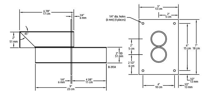
Figure 17: Typical Grinder Take-Off Attachment
